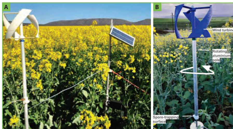
Figure 3: Two novel simplistic spore trap prototypes developed in collaboration with Dr André van der Merwe are displayed. In (A), both prototypes are present: Prototype 1 on the left and Prototype 2 on the right. The wind turbine atop Prototype 1 can be seen on the left and the solar panel powering the rotorods is visible on the right. In (B), the main structure of Prototype 1 is illustrated: A wind turbine attached to an aluminium pole that rotates as the wind blows, and an adhesive-coated acrylic rod that acts as the spore-trapping surface which ascospores, drifting in the air, stick onto.
